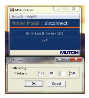
Change the IP address to the IP address of the printer in the LAN setting window and press "OK". (IP address displayed is for example only)
